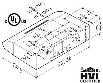
HVI-2100 CERTIFIED RATINGS comply with new testing technologies and procedures prescribed by the Home Ventilating Institute, for off-the-shelf products, as they are available to consumers. Product performance is rated at 0.1 in. static pressure, based on tests conducted in a state-of-the-art test laboratory. Sones are a measure of humanly-perceived loudness, based on laboratory measurements.
